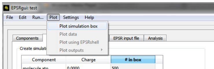
In the top menu bar, click Plot->Plot simulation box. The dialog window that opens gives options as to which atoms and how much of the box to plot.
