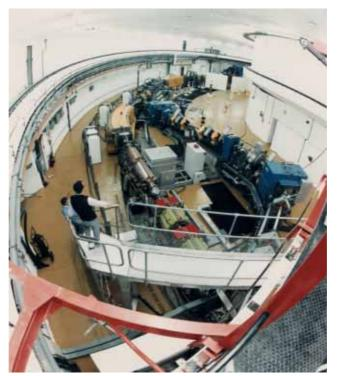
Electrons stripped from the H<sup>-</sup> ions. Resulting protons are accelerated to 800 MeV, and split into two bunches
