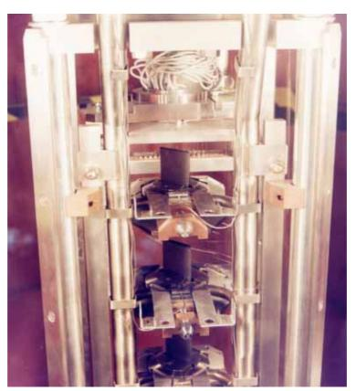
Carbon target, 10 mm thick Takes 2-3% of the proton beam
