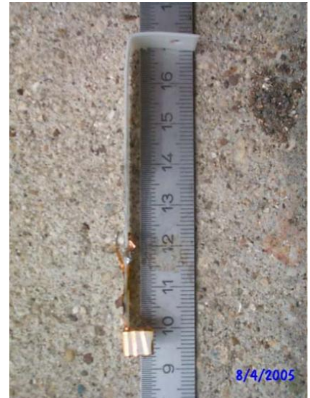
Copper foil coil wrapped round small sample (fly-past)
