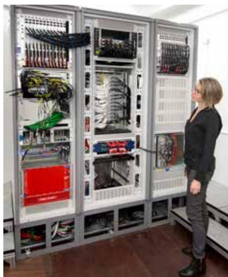
Fig. 5.5. Shows DAE rack installation for the MARI beamline
