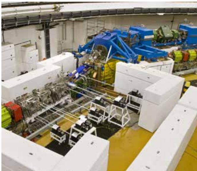
Fig. 3.12. Straight 1, enclosed by concrete shielding, where 'bad beam' is lost. The long horizontal rods are drive rods for the adjustable beam collectors incorporated in the beam line.
