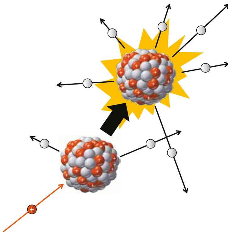
Fig. 2.1. Schematic representation of proton-induced spallation of a heavy nucleus giving rise to neutrons (shown in white).
