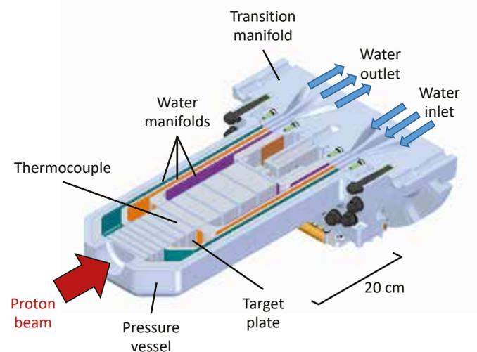
Fig. 3.16. Schematic diagram of TS-1 neutron-producing target.
