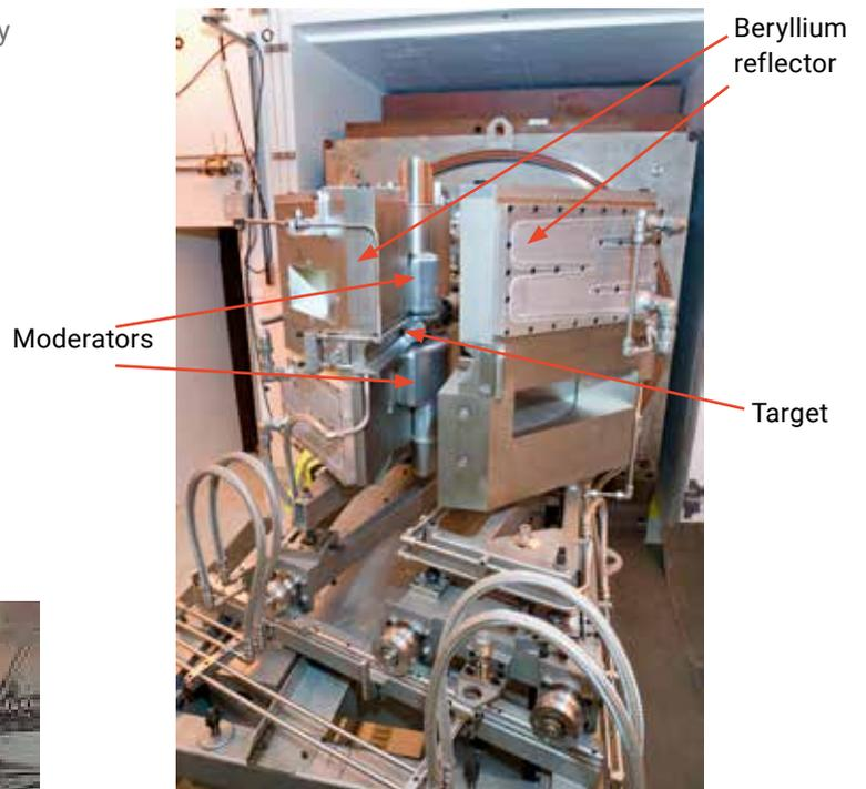
Fig. 3.19. TS-2 target, reflector and moderator assemblies.
