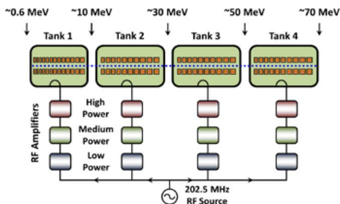
Fig. 3.8. Block diagram of linac and RF system. Feedback circuits necessary for successful operation are not shown in this diagram.
