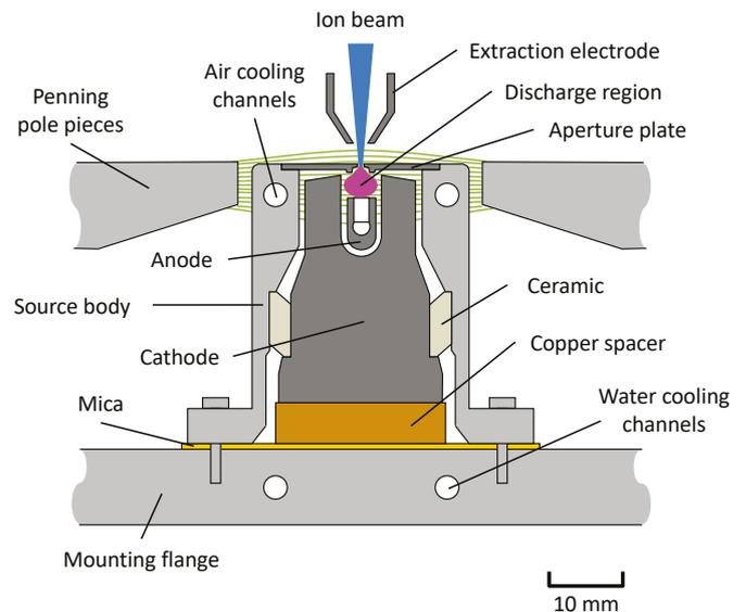
Fig. 3.3. A cross-section through the ISIS ion source. The discharge region is roughly the size of a peanut.
