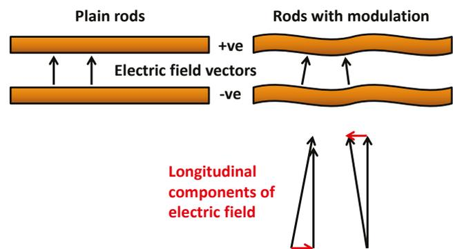
Fig. 3.4. Schematic illustration of electric fields between two RFQ rods. Left-hand side, focusing only; right-hand side, 'wiggles' create longitudinal component of electric field to accelerate and bunch particles.
