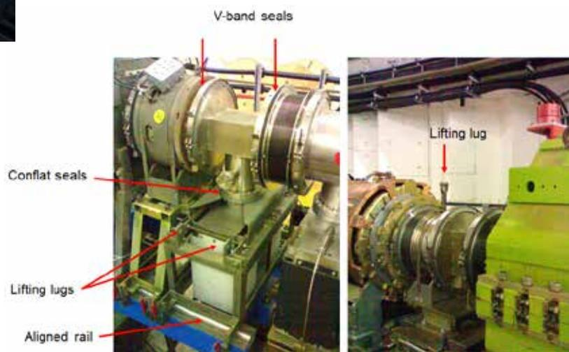
Fig. 4.2. Illustration of preparations for rapid replacement of a sub-assembly.
