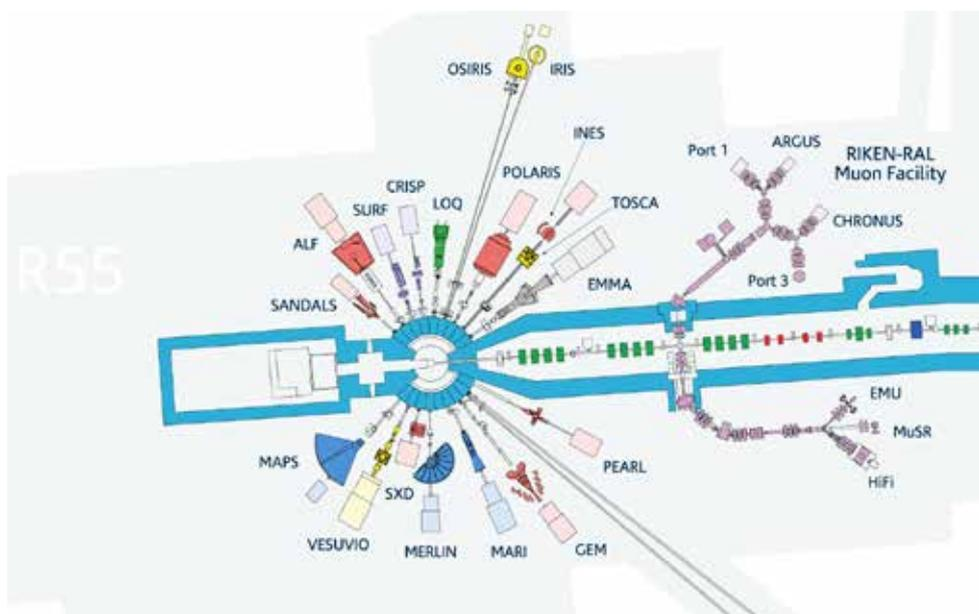
Fig. 5.3. Layout of instruments on Target Station 1. The two beam lines that continue past the foot of the diagram lead to Engin-X and HRPD.
