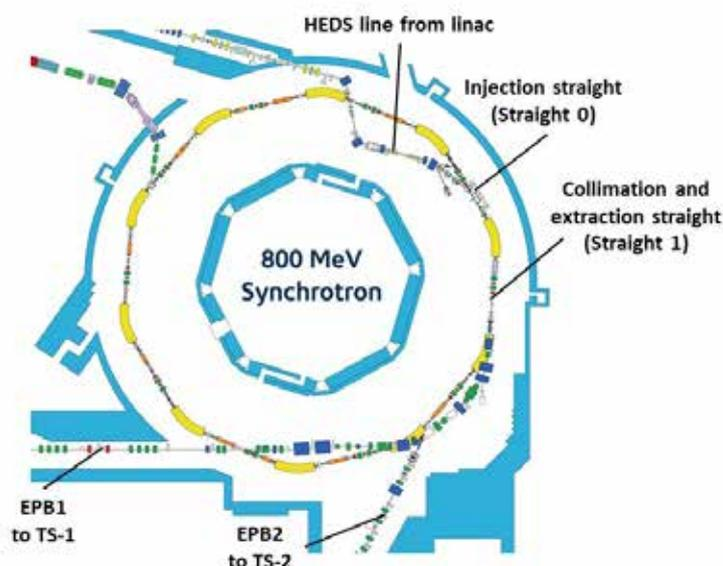
Fig. 3.9. Schematic diagram of the ISIS synchrotron. Yellow, dipoles; dark green, quadrupoles; red, trim magnets.
