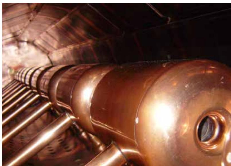
Fig. 3.7. The interior of Tank 3 showing the long line of drift tubes; each drift tube is supported by two legs and incorporates a 3 cm diameter hole through which the  $H^-$  beam passes. The upper half of the copper RF liner is in place in this photo.
