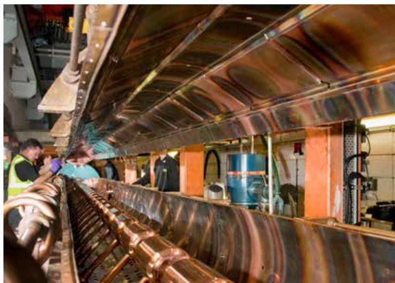
Fig. 3.6. Tank 3 with both the upper half of the steel vacuum vessel and the upper half of the copper RF liner removed.
