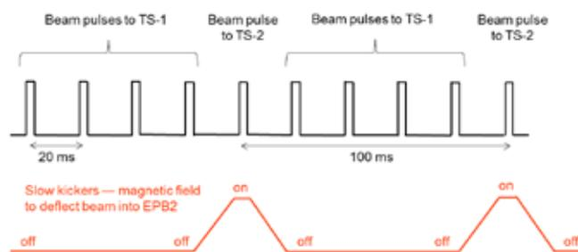
Fig. 3.13. Schematic representation of operation of slow kickers deflecting beam into EPB2. These kicker magnets are 'slow' because they have almost 20 ms to ramp up to full field and another 20 ms to ramp down, unlike the extraction kickers in the synchrotron that must switch on within  $0.1 \mu\text{s}$ .
