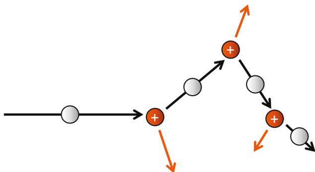
Fig. 2.2. Schematic representation of neutron moderation. Neutrons (white) undergo successive collisions with recoiling hydrogen atom nuclei (red), slowing them down. After some 14 collisions in hydrogen, neutrons with energies in the MeV region slow down to energies in the meV – eV region.
