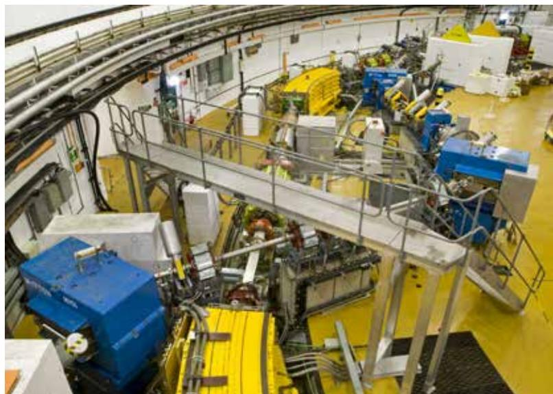
Fig. 3.11. HEDS line entering the synchrotron room. In this photograph, under the bridge, the HEDS line passes over the synchrotron orbit travelling from left to right.
