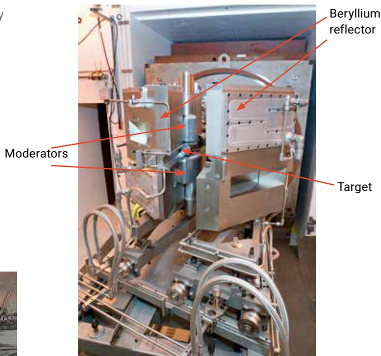
Fig. 3.19. TS-2 target, reflector and moderator assemblies.
