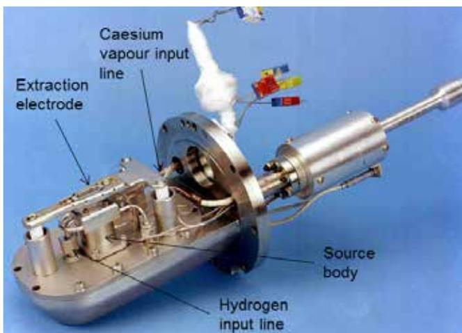
Fig. 3.2. The heart of the ISIS ion source assembly. The source body is shown in more detail in Fig. 3.3.
