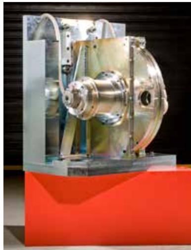
Fig. 5.2. Double disk neutron chopper for the Zoom instrument
