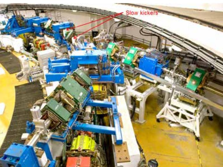
Fig. 3.14. Extracted proton beams EPB1 (on left-hand-side) and EPB2 (on right-hand side) leaving the synchrotron. One of the lattice quadrupoles (light green) and one of the trim quadrupoles (red) on the synchrotron orbit can be seen at the foot of the photograph.
