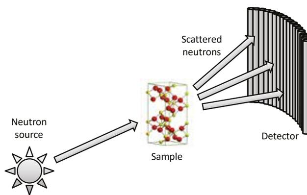
Fig. 2.3. Schematic representation of neutron scattering.
