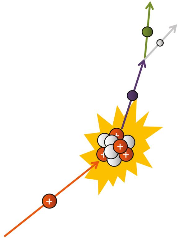
Fig. 2.4. Schematic representation of muon production. Protons (red) generate pions (blue) in a graphite target, which then decay to muons (green) and neutrinos (grey).
