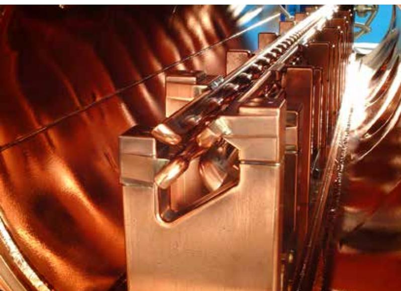
Fig. 3.5. The ISIS RFQ showing the four-rod assembly both outside and inside its copper-plated stainless-steel vessel. The four rods generate the quadrupole focusing field, and the modulations that gradually increase both in depth and in wavelength produce the bunching and acceleration.
