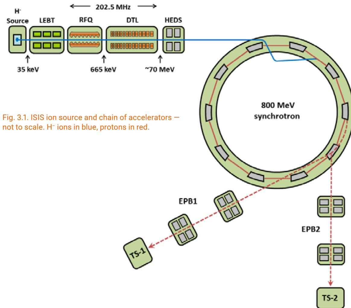
Fig. 3.1. ISIS ion source and chain of accelerators – not to scale.  $H^-$  ions in blue, protons in red.
