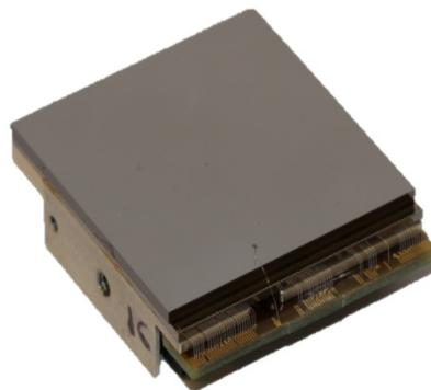
A HEXITEC detector module with 1mm thick CdTe mounted on the ASIC and mechanical block.
