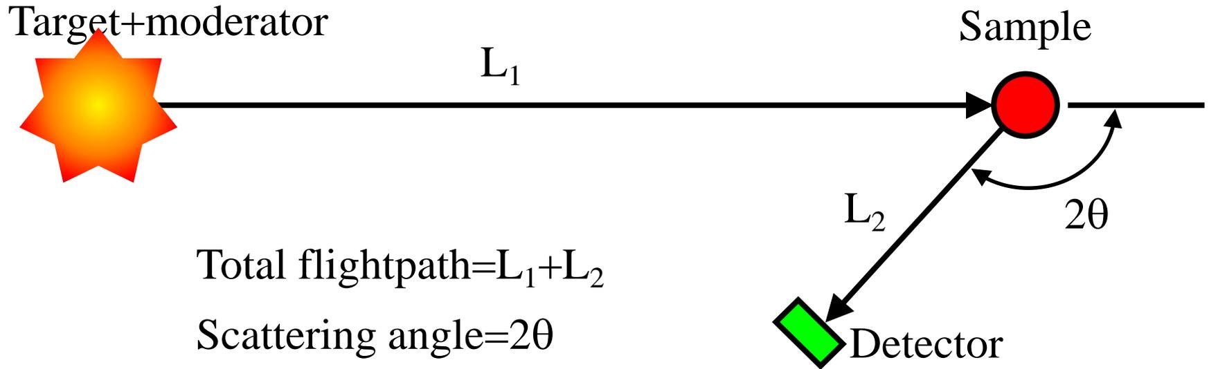
Measure time,  $t$ , taken by neutron to travel source to sample to detector
