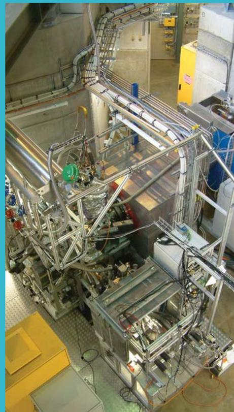
*The LEM facility at PSI. The mean implantation energy of the muons can be tuned from 1 keV to 3 keV corresponding to tunable implantation depths of a few nanometers to 100's of nanometers.*
