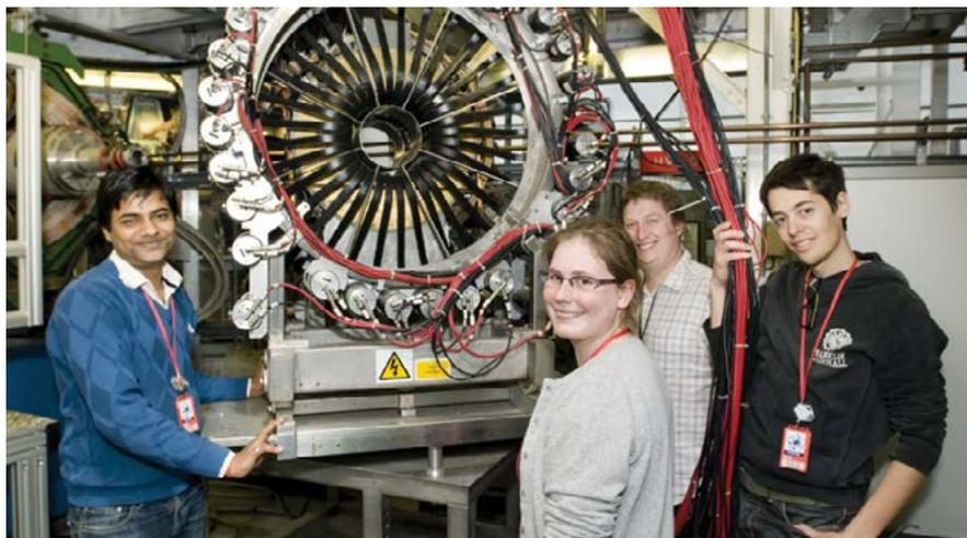
*The MuSR spectrometer at ISIS. The MuSR detectors can be rotated by 90° allowing measurements to be made in both longitudinal and transverse applied fields. Experiments can be performed from 30 mK to 1000 K.*
