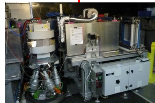
Heavy-duty hexapod for sample support
