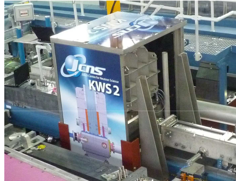
New double-disk Chopper 12,000 rpm, Disk diameter 620 mm
