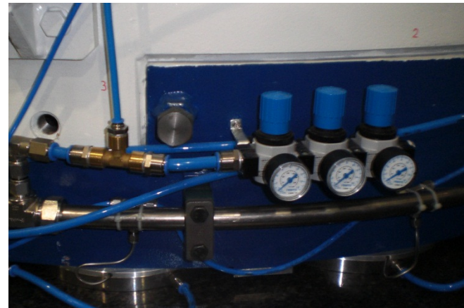
Air cushion feet for manual movement of the detector housing 12 t (weight)
