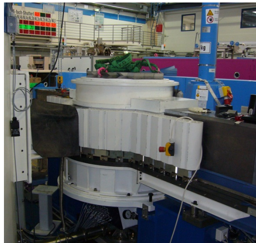
Monochromator burg with lead shielding curtain and air flight tube
