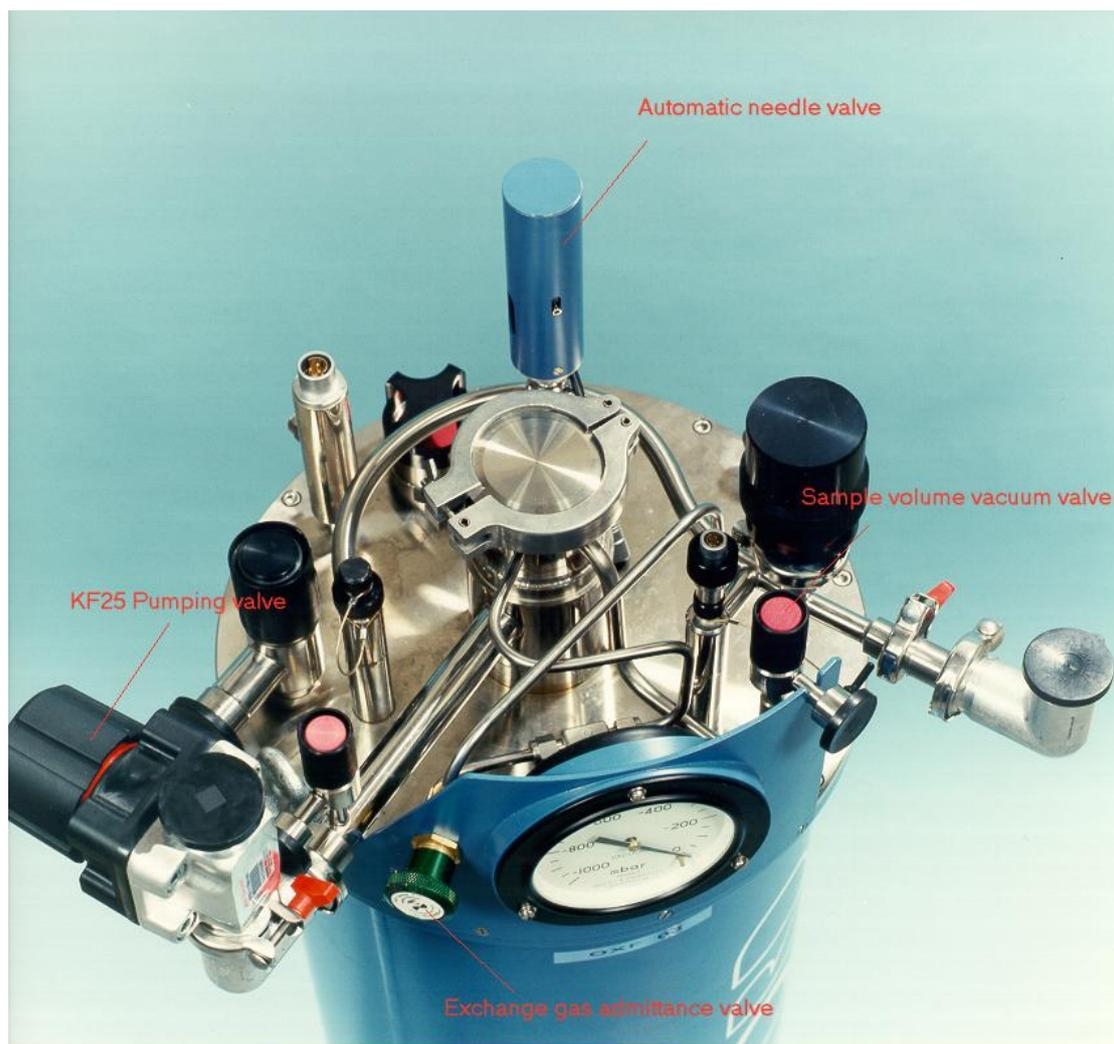
Turn on the pump and evacuate the line and **then** open the KF25 valve.
