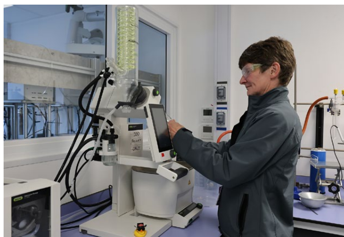
Rachel Pearce prepares the rotary evaporator in the Deuteration Laboratory
