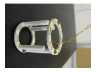
RF Coil: 'mouse size' saddle coil Tuned and matched to 50Ω between ~9-13MHz
