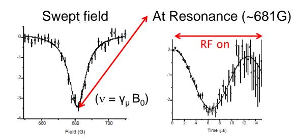
RF Coil tuned 9.2 MHz,  $(\gamma_{\mu} = 13.55 \text{kHz/G})$
