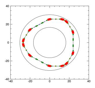
ISIS-II RCS Proposed Layout: A plan view of a proposed Rapid Cycling Synchrotron (RCS) design for ISIS-II showing the main dipole magnets in red and focusing quadrupoles and accelerating cavities in green and blue.
