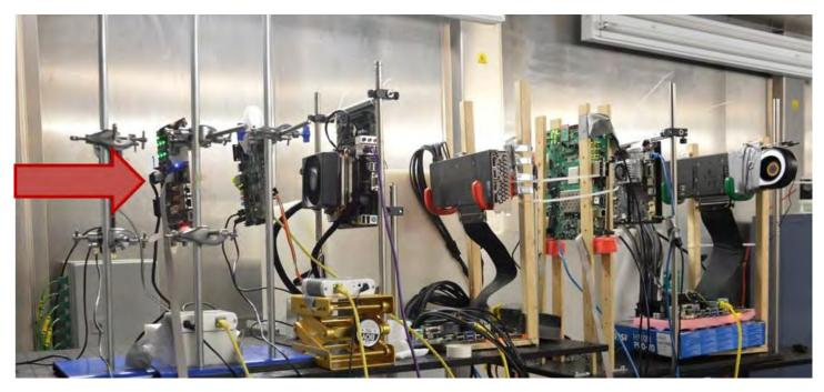
Electronic samples being tested in ChipIr.
