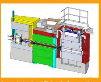
Cross-section through the ALFRed beamline (beam goes left to right) from choppers to entry into the blockhouse. The green area is currently a large void.
