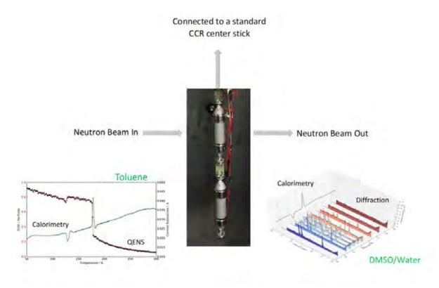
In-situ calorimetry + QENS cell set-up on IRIS. Left figure shows combined measurement of thermal transitions and elastic fixed window scan for toluene. Right figure shows combined measurement of thermal transitions with diffraction patterns for a DMSO/water mixture.
