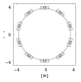
ISIS-II FFA Prototype Propose layout: A plan view of a proposed Fixed-Field Alternating-Gradient Accelerator (FFA) design for a small-scale prototype to prove the technology for a later potential full-scale ISIS-II design. Main bending magnets are shown in blue and red.
