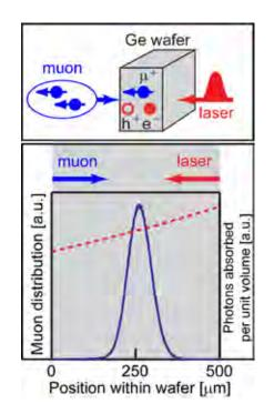
Top: Schematic diagram of the experimental geometry. Bottom: Muon distribution (blue solid line) and photon flux (red broken line) as a function of depth measured from the surface on which muons are incident. The muon distribution has been calculated using a Monte Carlo simulation package based on GEANT4. Credit: K Yokoyama.
