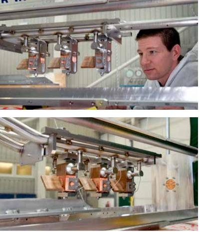
The muon target ladder, shown in Fig. 3.15, consists of three water cooled targets. Only one target is in the proton beam at any given time, but if one fails then a new one can be quickly inserted. Unlike at some other facilities the muon target is static (i.e. not rotating) and is edge cooled.
