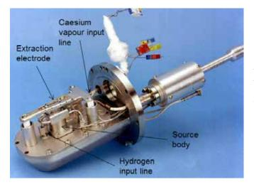
Fig. 3.2. The heart of the ISIS ion source assembly. The source body is shown in more detail in Fig. 3.3.
