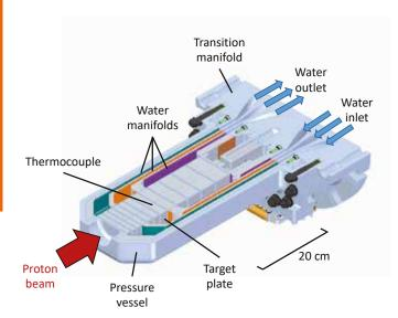
Fig. 3.16. Schematic diagram of TS-1 neutron-producing target.
