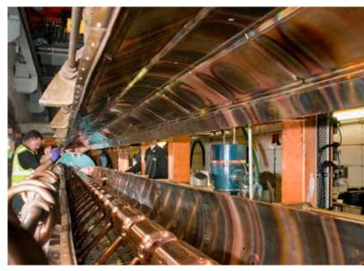
Fig. 3.6. Tank 3 with both the upper half of the steel vacuum vessel and the upper half of the copper RF liner removed.
