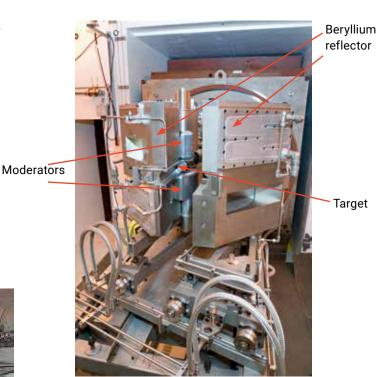
Fig. 3.19. TS-2 target, reflector and moderator assemblies.
