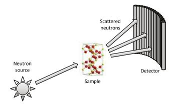
Fig. 2.3. Schematic representation of neutron scattering.
