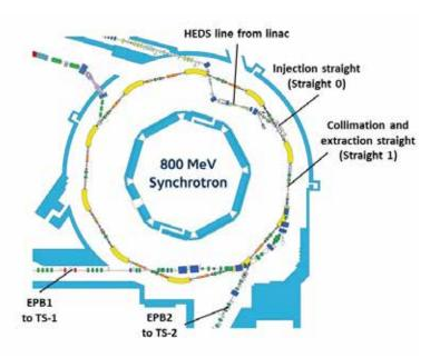
Fig. 3.9. Schematic diagram of the ISIS synchrotron. Yellow, dipoles; dark green, quadrupoles; red, trim magnets.
