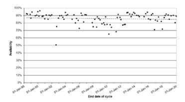
Fig. 4.3. Availability of the ISIS machine since 1998; the average is 86% with a standard deviation of 8%. Availability is defined simply as (number of beam pulses delivered to targets) ÷ (number of pulses scheduled to be delivered); ISIS counts every lost pulse as a lost pulse. Very roughly, ~75-80% of the down-time can be ascribed to the accelerators and their ancillary equipment, and ~20-25% to the target systems.
