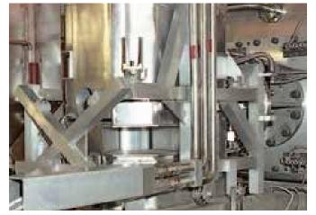
Fig. 3.17. TS-1 target, reflector and moderator assemblies.
