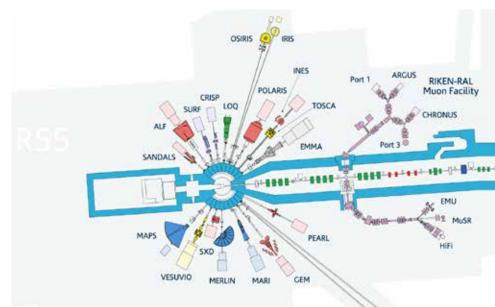
Fig. 5.3. Layout of instruments on Target Station 1. The two beam lines that continue past the foot of the diagram lead to Engin-X and HRPD.
