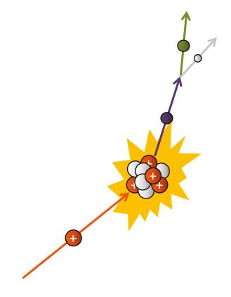
Fig. 2.4. Schematic representation of muon production. Protons (red) generate pions (blue) in a graphite target, which then decay to muons (green) and neutrinos (grey).
