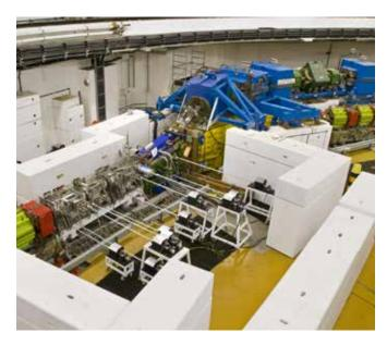
Fig. 3.12. Straight 1, enclosed by concrete shielding, where 'bad beam' is lost. The long horizontal rods are drive rods for the adjustable beam collectors incorporated in the beam line.
