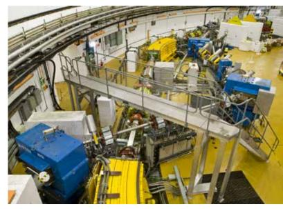
Fig. 3.11. HEDS line entering the synchrotron room. In this photograph, under the bridge, the HEDS line passes over the synchrotron orbit travelling from left to right.
