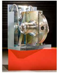
Fig. 5.2. Double disk neutron chopper for the Zoom instrument
