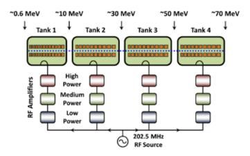
Fig. 3.8. Block diagram of linac and RF system. Feedback circuits necessary for successful operation are not shown in this diagram.
