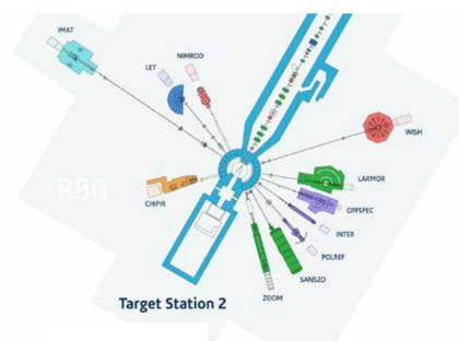
Fig. 5.4. Layout of instruments on Target Station 2.
