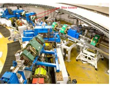
Fig. 3.14. Extracted proton beams EPB1 (on left-handside) and EPB2 (on right-hand side) leaving the synchrotron. One of the lattice quadrupoles (light green) and one of the trim quadrupoles (red) on the synchrotron orbit can be seen at the foot of the photograph.
