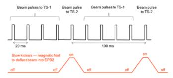
Fig. 3.13. Schematic representation of operation of slow kickers deflecting beam into EPB2. These kicker magnets are 'slow' because they have almost 20 ms to ramp up to full field and another 20 ms to ramp down, unlike the extraction kickers in the synchrotron that must switch on within 0.1  $\mu$ s.
