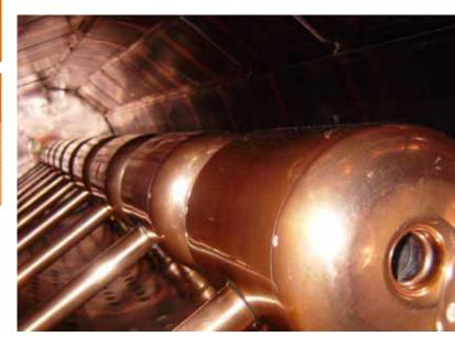
Fig. 3.7. The interior of Tank 3 showing the long line of drift tubes; each drift tube is supported by two legs and incorporates a 3 cm diameter hole through which the H<sup>-</sup> beam passes. The upper half of the copper RF liner is in place in this photo.
