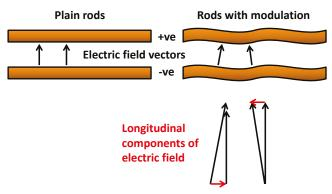
Fig. 3.4. Schematic illustration of electric fields between two RFQ rods. Left-hand side, focusing only; right-hand side, 'wiggles' create longitudinal component of electric field to accelerate and bunch particles.
