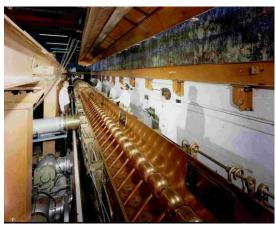
Next, the bunched beam enters the 40-metre long Linear Accelerator (Linac) which consists of many tube-shaped electrodes inside electrical resonator tanks. The linac accelerates the beam up to 37% of the speed of light.
