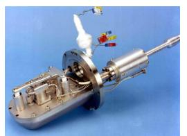
It all starts at the Ion Source. Hydrogen gas and caesium vapour are fed into a space the size of a peanut and, after the application of a 50 amp electric discharge,  $H^-$  ions (a proton with two electrons) are produced.
