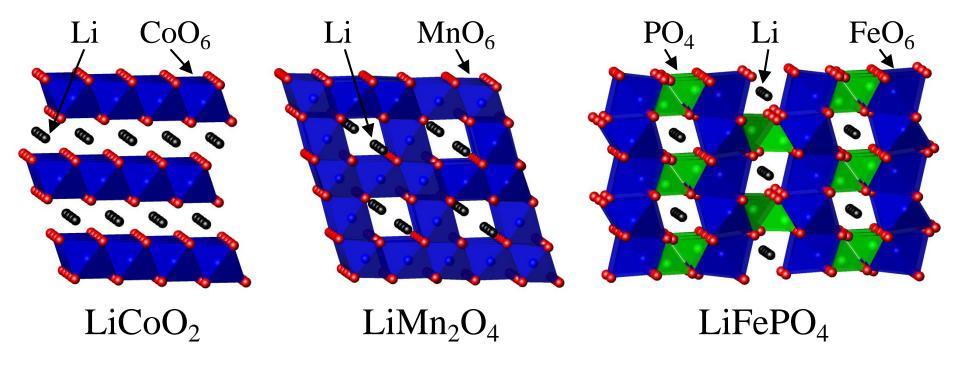
From a crystal structure point-of-view, ease of lithium removal/ insertion is facilitated by Li layers (LiCoO<sub>2</sub>) or Li channels (LiMn<sub>2</sub>O<sub>4</sub> and LiFePO<sub>4</sub>).
