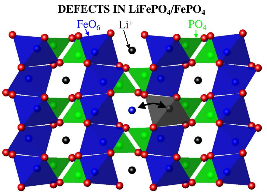
Concentration of anti-site defects is low (few %)  $\Rightarrow$  at limit of method. But they are a factor in capacity fade on repeated charge/discharge.
