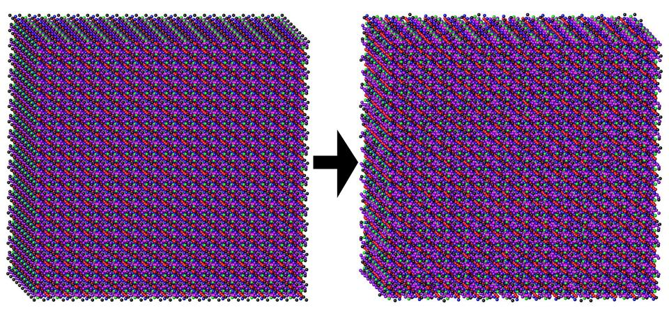
In this case :  $9 \times 14 \times 17$  unit cells of LiFePO<sub>4</sub> (total of 59976 atoms). Move atoms to fit neutron total scattering data (wide *d*-spacing range). Analyse final configuration to probe local atom-atom correlations, *etc*.
