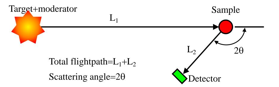
Measure time, *t*, taken by neutron to travel source to sample to detector  $\Rightarrow$  velocity,  $v=(L_1+L_2)/t \Rightarrow$  energy,  $E=\frac{1}{2}mv^2$ , *m* is the neutron's mass. Also, energy,  $E=\frac{h^2}{2m\lambda^2}$ , where *h* is Planck's constant.
