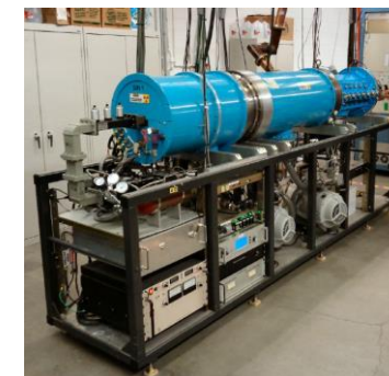
The NT 30 mA DC H + accelerator achieves proton energies of 1.85 – 2.6 MeV for research applications
