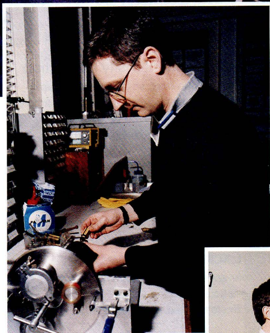
Above: Richard Todd (UMIST) mounts his ceramic composite sample in order to measure residual stress on HRPD. [96RC1260]
