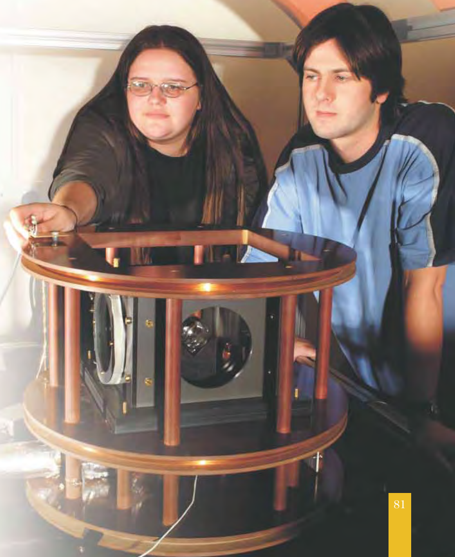
Fig. 3.10. Kathryn Baker and Steven Parnell setting up the spin-exchange apparatus in the new optical pumping laboratory at ISIS (02EC3168).
