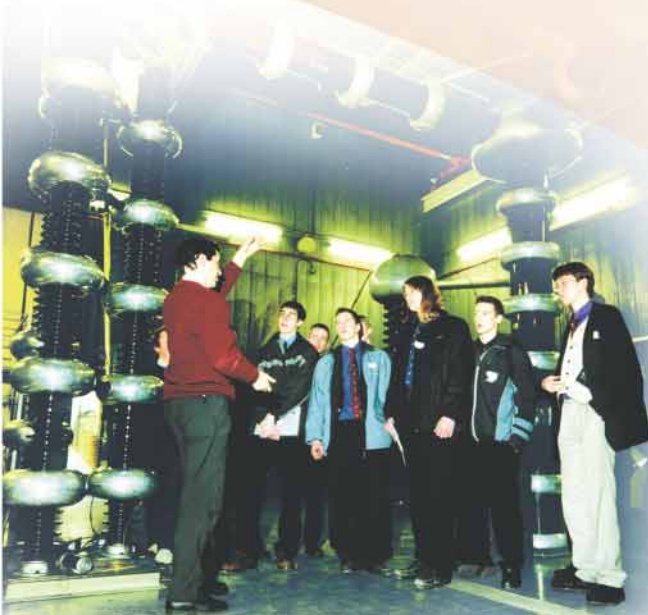
John Thomason (ISIS) explains the workings of the Cockcroft-Walton pre-injector to A-level students attending the Oxford Particle Physics Masterclass (02RC1583).
