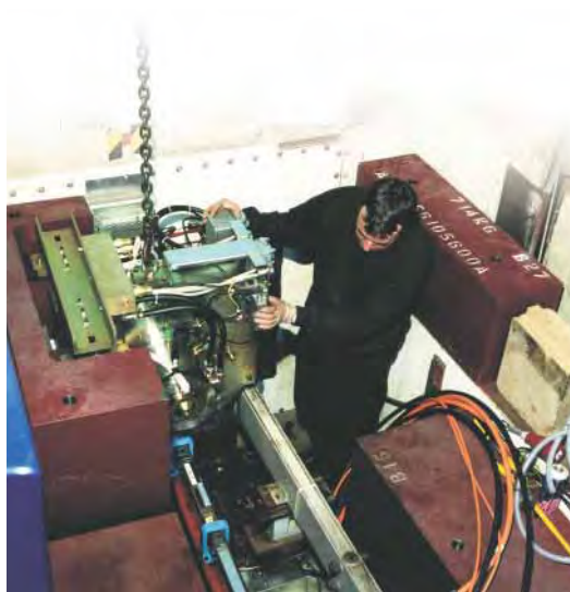
Fig. 5.17. Mike Brind installing the new counter-rotating chopper on ENGIN-X (02RC2729).
