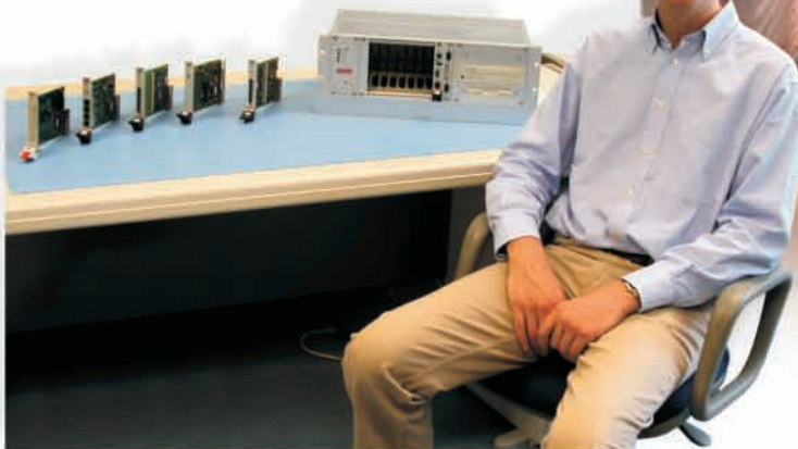
Fig. 27: Clive Lambourne of the Controls Group with the compact PCI system intended to replace the present STEbus system.
