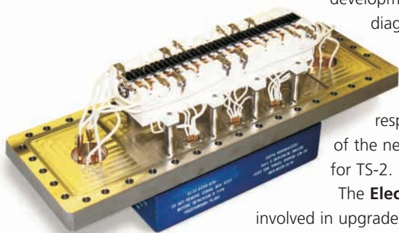
A new gas ionization beam profile monitor for the synchrotron ring. The 40 individual channeltron detectors in the monitor will allow instantaneous measurement of the horizontal beam profile.
