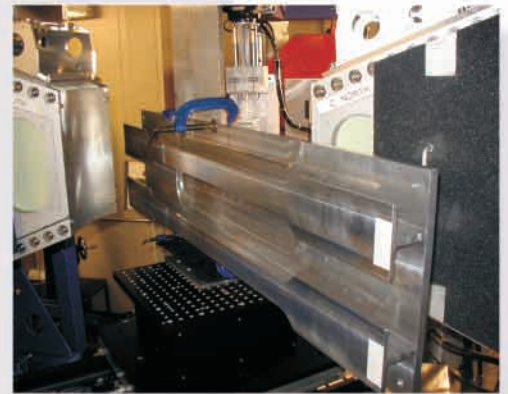
A structural-scale aircraft test panel in place on the ENGIN-X instrument.
