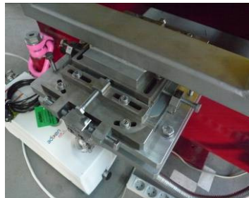
4 adjustment units for precision positioning
