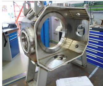
4 UHV pump boxes with complicated geometry
