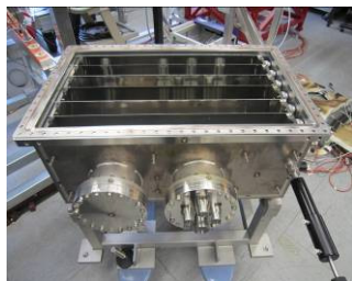
NEG-pump system with 10 NEG-pumps and heat protection jalousie
