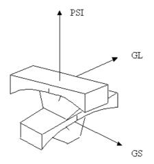
**Figure:** Definition of the goniometer arcs. Positive rotations of both GS and GL are shown.
