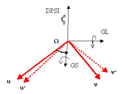
Note that u and v are not necessarily perpendicular. The misorientation is described by rotations performed in the following order:
