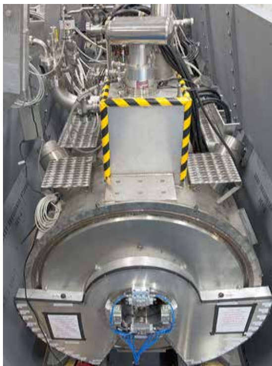
MICE employed a 12-coil superconducting solenoid assembly combining large apertures with strong magnetic fields to contain and focus the highly divergent muons.
