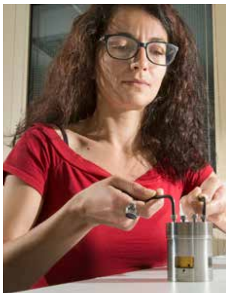
Left: PhD student Mara Capone with the high-pressure cell currently being developed for use on the PEARL diffractometer.
